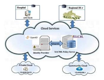
Figure 1. Common identity management and access control method deployed as cloud service.
