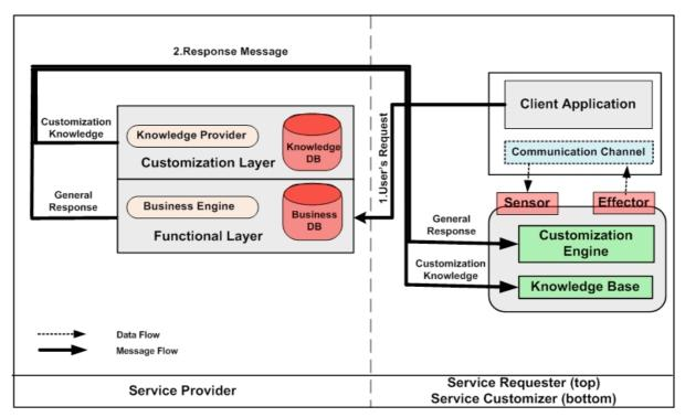
Figure 3. Proposed architecture: the client application sends a request message to the service provider; the service provider employs the service customizer to personalize its general service responses for the client.
