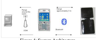
Figure 4: System Architecture
