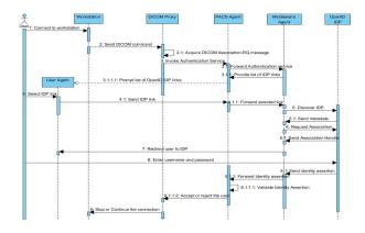
Figure 2. Sequence diagram for authentication of a user, compatible with OpenID protocol.
