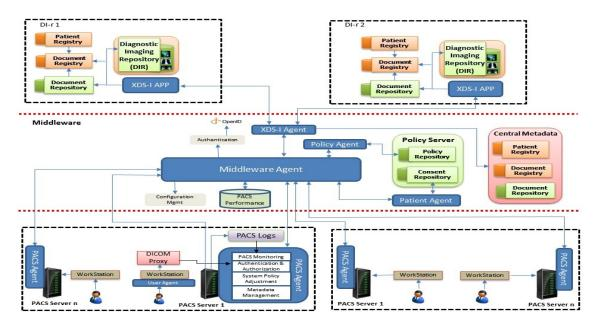
Figure 1. Overall view of the proposed infrastructure to make a secure and seamless connection between the DI-r and PACS systems. Each PACS server is supported by a generic agent called PACS Agent.
